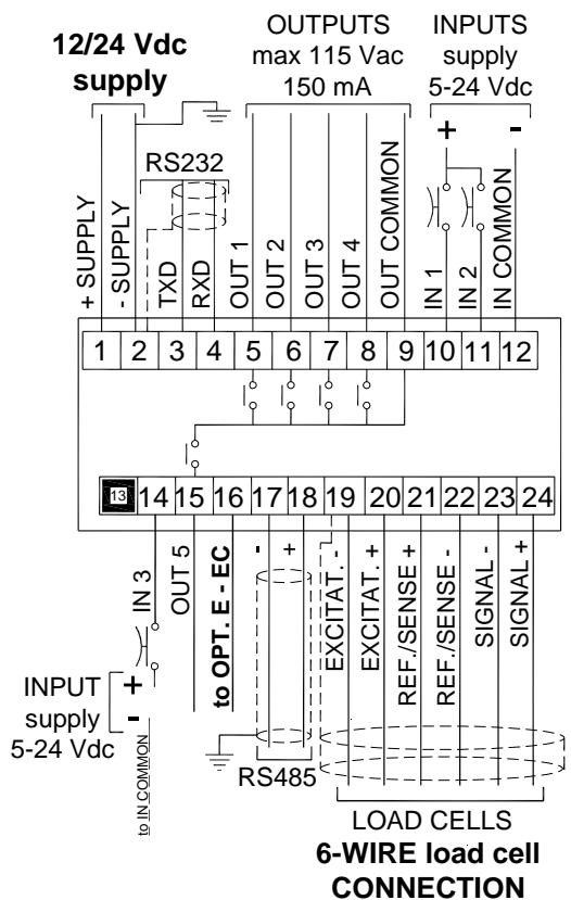
**5 outputs:** settable setpoint or remote output management via protocol.
